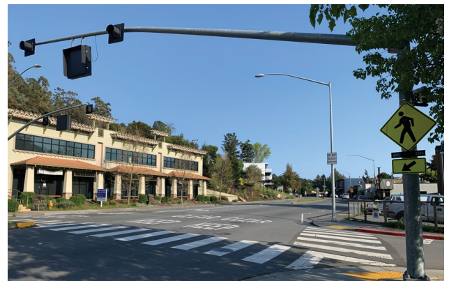
Street crossing with striping and beacons
