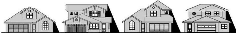
These second stories held toward the center of the property allow greater sunlight into neighboring properties and help protect views and privacy.
