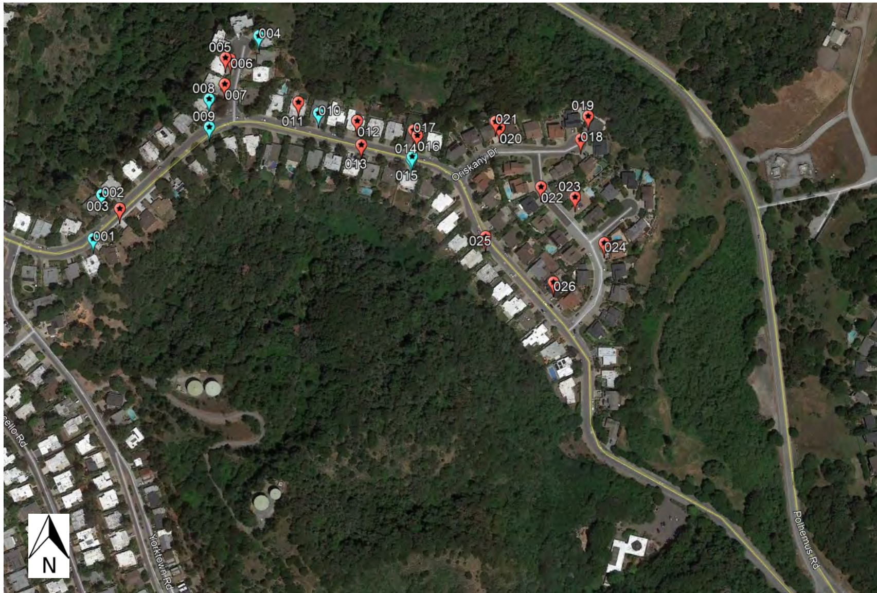
Figure 4: Basin CS-10 Area Defects (Blue star: Smoke testing form pages 1 & 2 completed. Red star: Standard cleanout. Smoke testing form page 2 completed)
