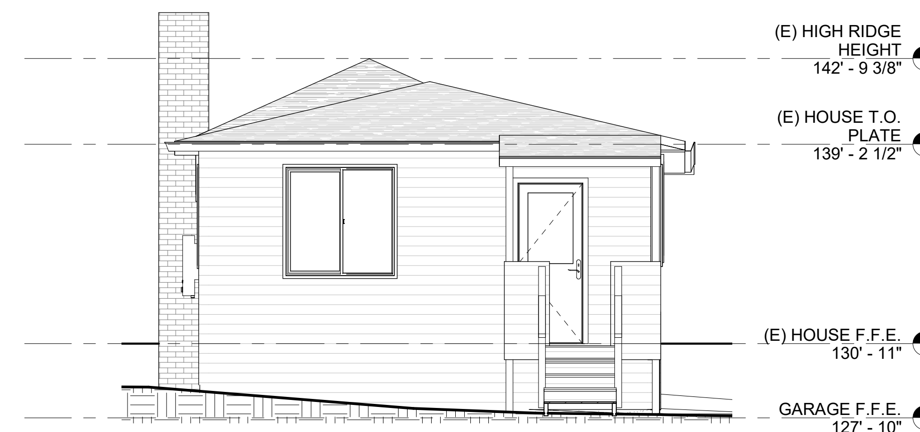
③ EXISTING REAR ELEVATION 1/4" = 1'-0"
