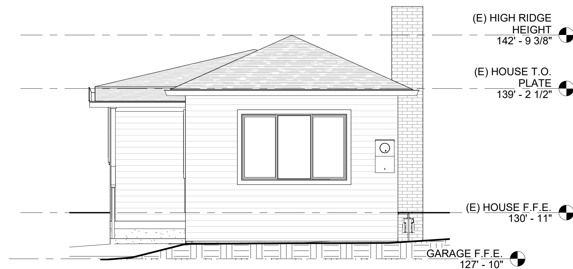
① EXISTING FRONT ELEVATION 1/4" = 1'-0"
