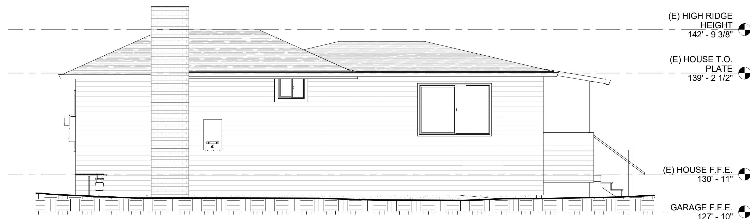
④ EXISTING RIGHT SIDE ELEVATION 1/4" = 1'-0"
