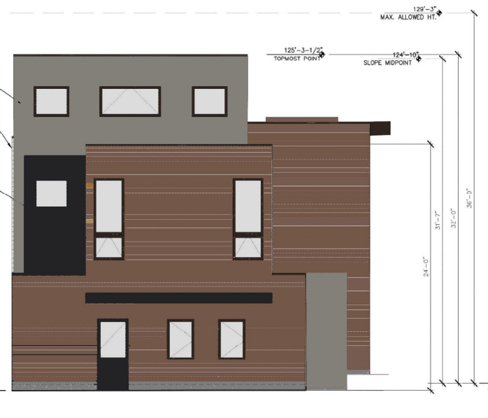
③ EAST EXTERIOR ELEVATION 1/4"=1'-0"
