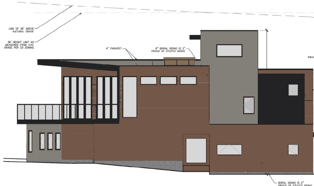
④ SOUTH EXTERIOR ELEVATION 1/4"=1'-0"
